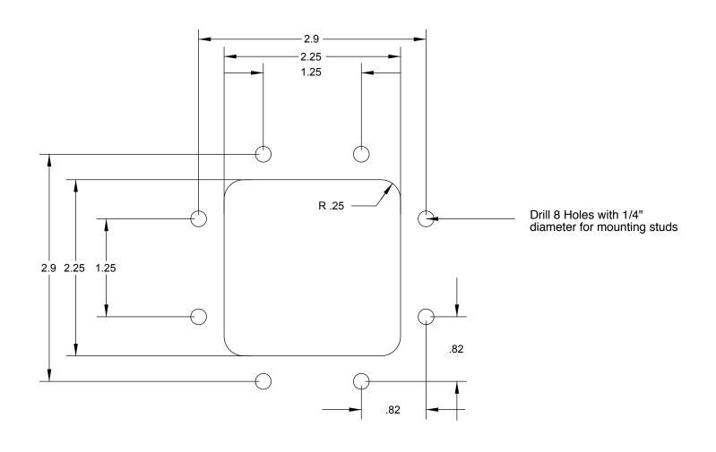
2" Window Body Overall Dimensions: 3" x 3" Reinforcement Plate Overall Dimensions: 3 3/8" x 3 3/8"
