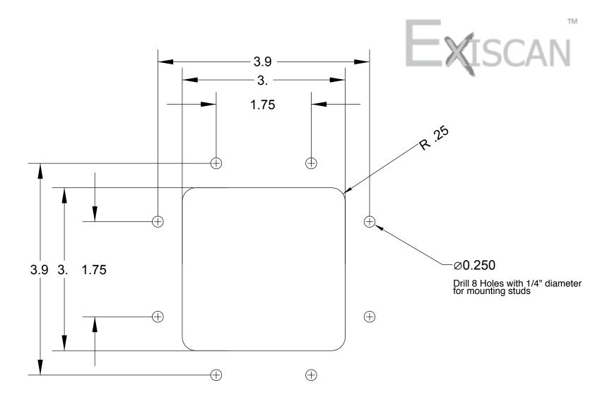
3" Window Body Overall Dimensions: 5" x 5" Reinforcement Plate Overall Dimensions: 5 3/8 x 5 3/8 MP1001Rev 1 1/14/15 Exiscan, LLC
